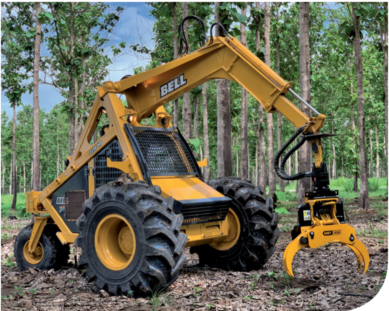
Bell Equipment logger with a GMT C10 quick coupler and GMT035 grapple saw
